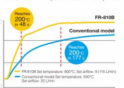
\* Examination of time taken for connector sections soldered onto a ceramic board to be heated to 200°C with maximum temperature and airflow settings selected. Single nozzles with an approximately 4mm diameter were used.
